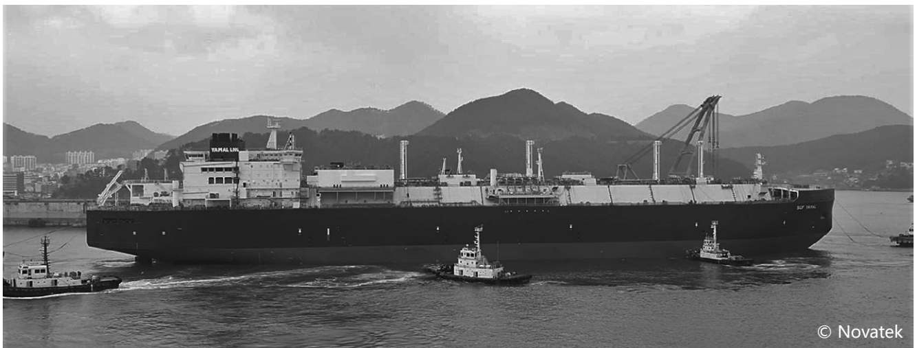
Ships servicing Port Sabetta require a channel that's around 300 metres wide and 15 metres deep
