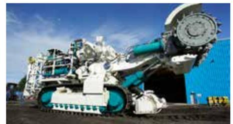
*Nautilus Minerals' "Bulk Cutter" for fragmenting the seabed before another machine collects it (Image © Nautilus Minerals)*
